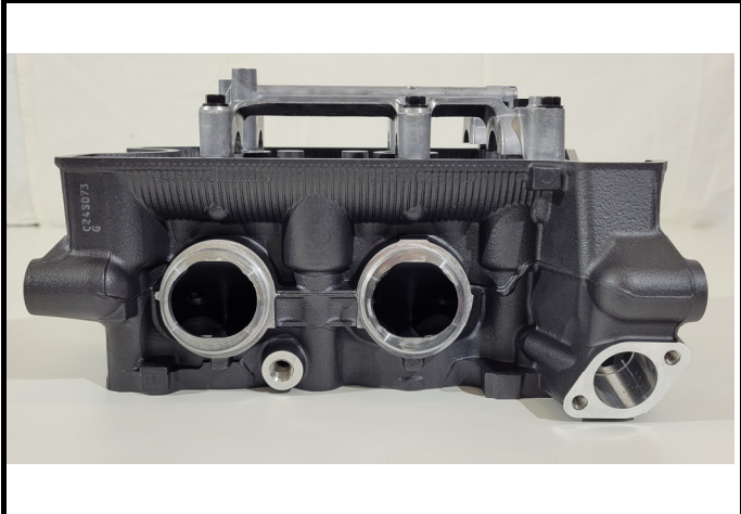
C8-3) Culasse nue vue côté admission Bare cylinderhead seen from intake side
