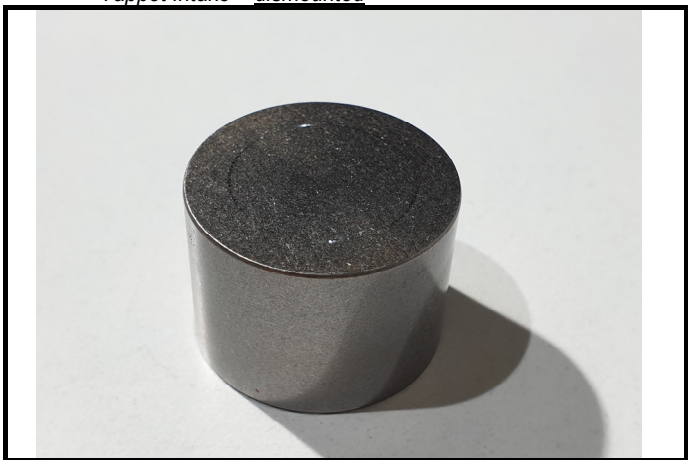
C10-6) Poussoir Admission – démonté Tappet Intake – dismounted
